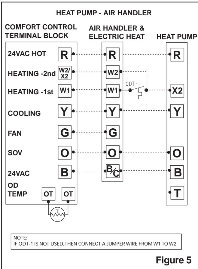
8. Match and connect control wires to proper terminals on the connector block. (See figures 3, 4 & 5).
